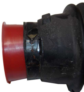
Figure 6: Red Plug Start of engagement into firewall connector
