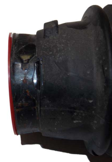
Figure 7: Red Plug Fully installed into firewall connector.
