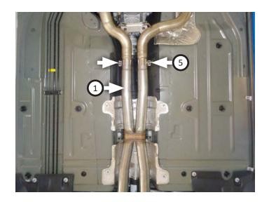
7. Place (x2 ea.) clamps (6) onto each muffler (2) then connect them to scavenger outlets. Level mufflers and tighten clamps just enough to allow for adjustment.
