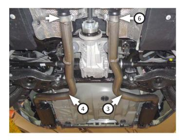
9. Replace ground strap (removed step 4) onto hanger on right tailpipe.
