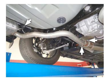
4. Support right side muffler and loosen clamps at slip fit connections behind catalytic converters. Unclip ground strap from middle hanger then slide system off of head pipes and set it aside.
