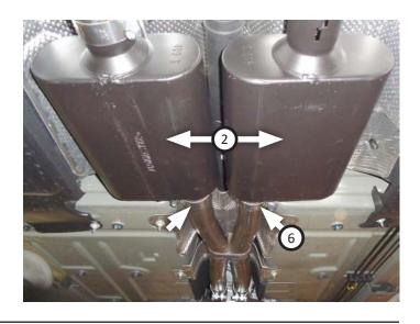
8. Place (x2) clamps (6) onto left (3) and right (4) tailpipes then connect them to mufflers. Level tailpipes and center tips in exhaust bezels; insert wire hangers in isolators and tighten clamps loosely.
