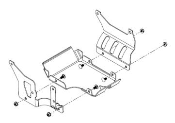
2. Bolt the shield assembly onto oil pan using the M8 x 16 Flange Head Bolts, leaving them finger tight.
