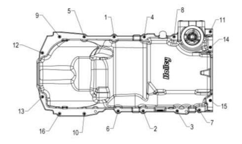
Torque: M8 bolts to 18 ft./lbs. (bolts 1 through 13, and 16) M6 bolts to 106 in./lbs. (bolts 14 and 15)
