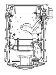
**IMPORTANT:** While the bolts are started, but still loose, lift the pickup tube. Tighten the two bolts while maintaining the lifted position. This process ensures proper clearance between the pickup inlet and the pan floor.
